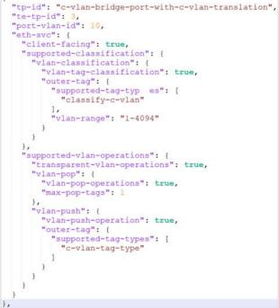
Figure C.2.2.1.1: Ethernet LTPs for C-VLAN Bridged Networks
