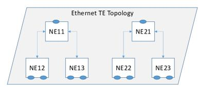
Figure 4.3.3.2.1.1: AL2 Ethernet Topology: Partial Connectivity, VLAN Isolation
