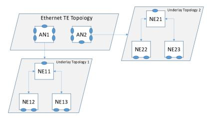
Figure 4.3.3.2.3.1: AL2 Ethernet Topology: Partial Connectivity, Use of Underlays
